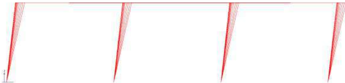
Figura 32a - Deformata SLV (+y) c.f.1
